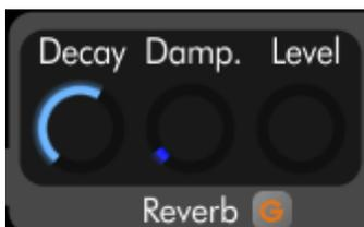
You can add a simple to configure but high-quality reverb effect to each slot. To deactivate the reverb, just keep the „level“ setting on the left position.
