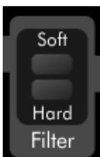
In this section you can choose between a 18 dB/oct (soft) or 24dB/oct (hard) filter or disable the filter at all. Cutoff, Reso, EnvMod and Emphasis is only available in filter mode.
