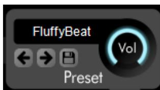
Groovestar 3.0 has an own preset manager. You can store your current settings in a preset by clicking on the „disc“ button shown above and choosing a file into which the settings should be stored.
