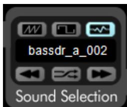
The sound selection field allows you to select a synthesized SAWTOOTH sound, a SQUARE sound or even a sampled WAVE file by engaging one of the three buttons above the sample name display:
